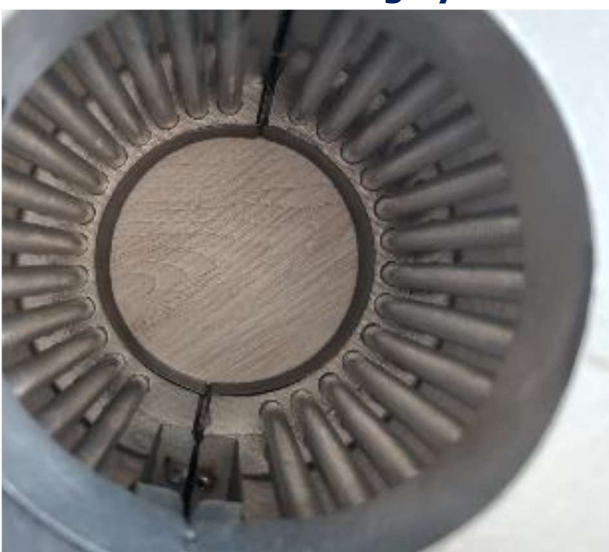
BKT's infrared heating system for the injection unit.
