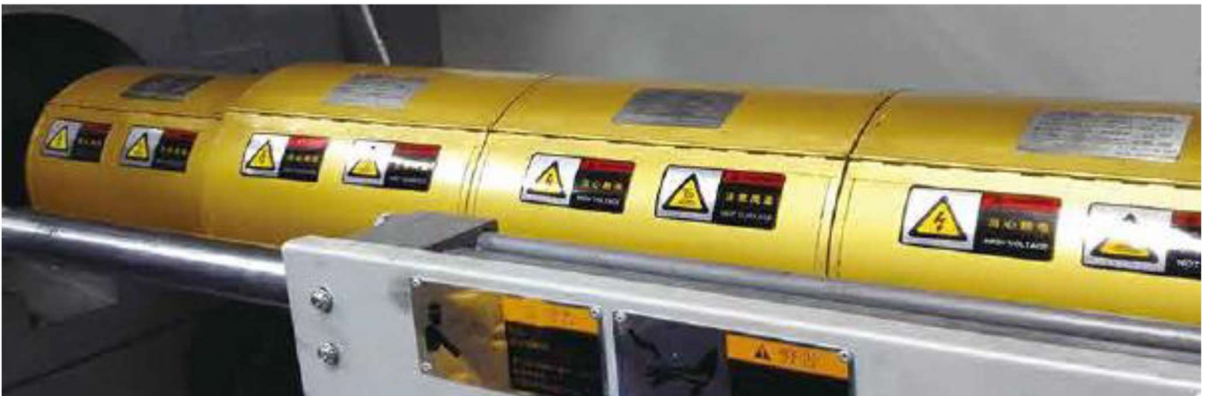
BKT's infrared heating system for the injection unit.
